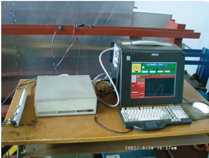
Fig. 5. A view of the Keithley P500 station cooperating with a microcomputer – the panel of software which allows to control the trailer systems, rolling speed and normal load of the trailer wheels
